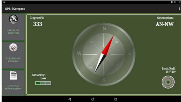
The Accuracy reading is for your reference. When the application determines that calibration is needed, it will pop up the “Calibration” graphics asking you to calibrate the compass. Hold the device and swing it in the way as shown on the screen. Do this several times until the popup graphics disappear.
