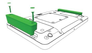
Fasten the Status Light to the I-Series 2.0 using the included screws and screw covers
