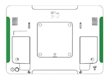
Remove the Edge Connect peripheral covers to expose the peripheral bay. Up to two Status Lights can be installed on a single I-Series 2.0 display.
