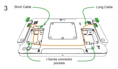
For cable routing, use cable clips (included in the box). An example of cable routing shown below:
