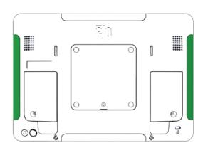
Remove the Edge Connect peripheral covers to expose the mounting interface. Up to two status lights can be installed on a single I-Series 2.0 display.
